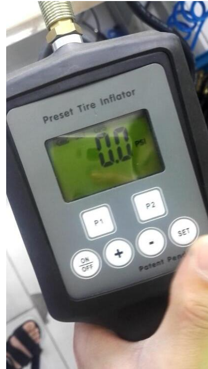
2. Press "SET" twice. "OPS" flashes on screen.
